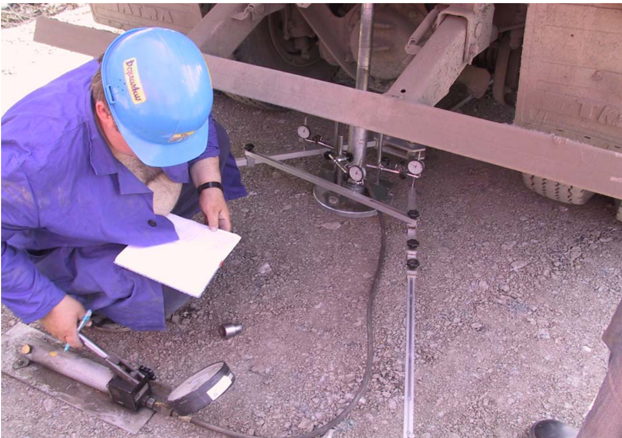
Fig. 7 Brestovany – Leopoldov, static loading test of the earth subgrade
